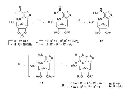
Scheme 2. Reagents and conditions: (a) hydrazine monohydrate/EtOH (2:1, v/v), reflux; (b) NaNO<sub>2</sub>, 10% acetic acid in H<sub>2</sub>O, 0 °C, 20 min, 71% from 8; (c) (i) TFA/H<sub>2</sub>O = 9:1, rt, 1 h; (ii) Ac<sub>2</sub>O, pyr, rt, 1 h, 73% from 10; (d) 10 equiv BnOH, xylenes, reflux, 5 h, 51%; (e) 10% Pd/C, H<sub>2</sub>, MeOH, rt, 90 min; (f) glyoxal or 2,3-butandione, EtOH, rt; (g) NH<sub>3</sub>/MeOH, rt, 1 h.
