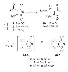
Scheme 1. Reagents and conditions: (a) hydrazine monohydrate, EtOH, reflux; (b) NaNO<sub>2</sub>, 10% acetic acid in H<sub>2</sub>O, 0 °C, 30 min; (c) ROH, xylenes, reflux, (d) 10% Pd/C, H<sub>2</sub>, MeOH, rt, 90 min; (e) 40% wt glyoxal, EtOH, rt.
